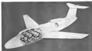
Four-engine turboprop transport would carry six passengers plus pilot. Seats, lavatories and baggage compartment are shown in cutaway.
